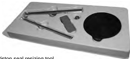
PTFE Piston seal resizing tool.
